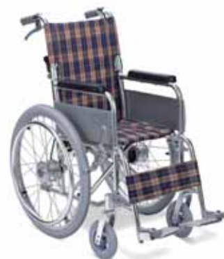
KL874LAH-30 CHILDREN TYPE, ALUMINUM CHAIR FRAME, FIXED ARMREST, FIXED FOOTREST, SOLID CASTOR, PNEUMATIC REAR WHEEL, DROP BACK HANDLE WITH DRUM BRAKE
