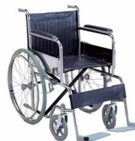
KL873 CHROMED STEEL FRAME, POWDER COATING CROSS BAR, FIXED ARMREST, FIXED FOOTREST, SOLID CASTOR, SOLID REAR WHEEL.
